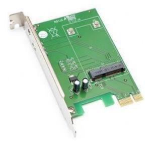
RouterBOARD 11E miniPCI-e to PCI-e Adapter for using four miniPCIe cards inside regular PC with PCI-e slots. Doesn't require any drivers. Note that this adapter doesn't support 3G modems, and doesn't have a SIM slot. For wireless cards only. **Product Specification**
